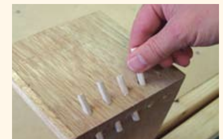
▼ Create the box. Insert dowels, cut to length and sand flush for a strong yet interesting mitred joint.
