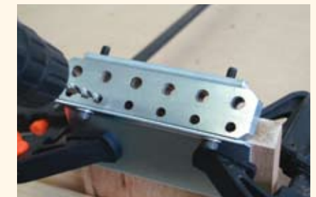
▼ Reinforce a mitre joint. Using the supplied 45 degree plate drill the holes through the mitre.
