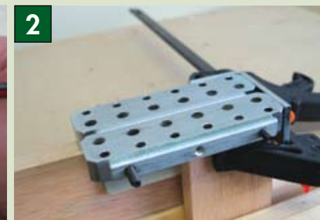
▼ Set-up. Place the two work pieces face side in, against the spacer plate and butt the edge of the timber against the stop plate.
