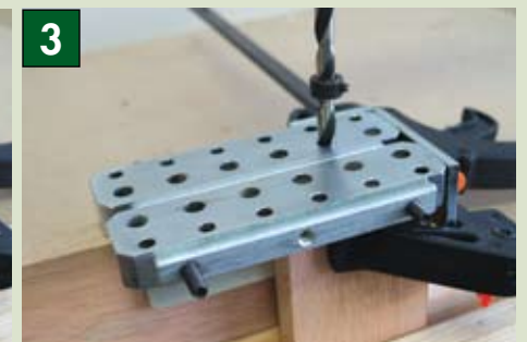
▼ Clamp and drill. With the work pieces firmly clamped to the base plate, drill the number of holes required on both pieces.
