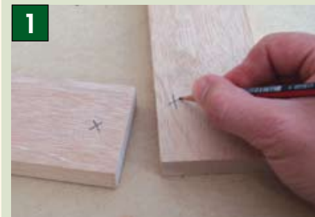
▼ Mark-up. The first step is to mark the face side of the timber and the face that will be joined. There is no need to measure.
